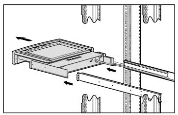
Figure 2-14. Removing the retractable tray from the rack
